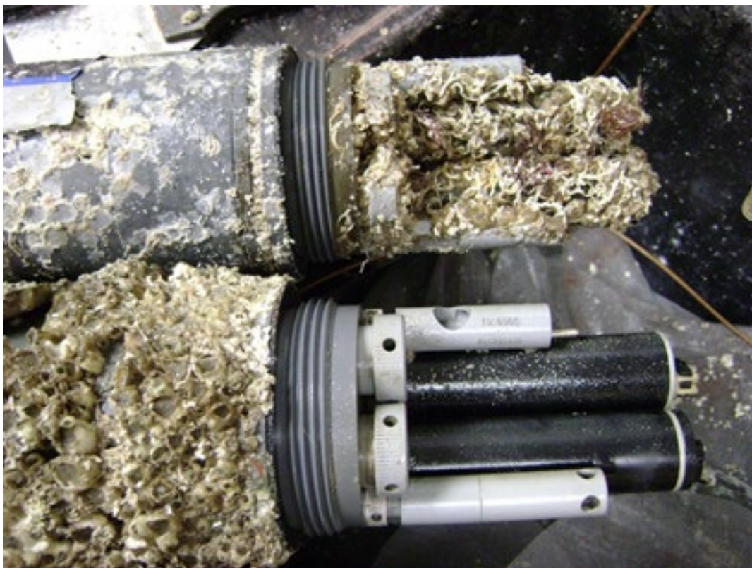
TWO WATER QUALITY INSTRUMENTS DEPLOYED SIDE BY SIDE SHOWING THE EXTENT OF BIOFOULING WITHOUT THE INVENTION (ABOVE) AND WITH THE INVENTION (BELOW). (SOURCE: JOE MEIMAN, NPS)
