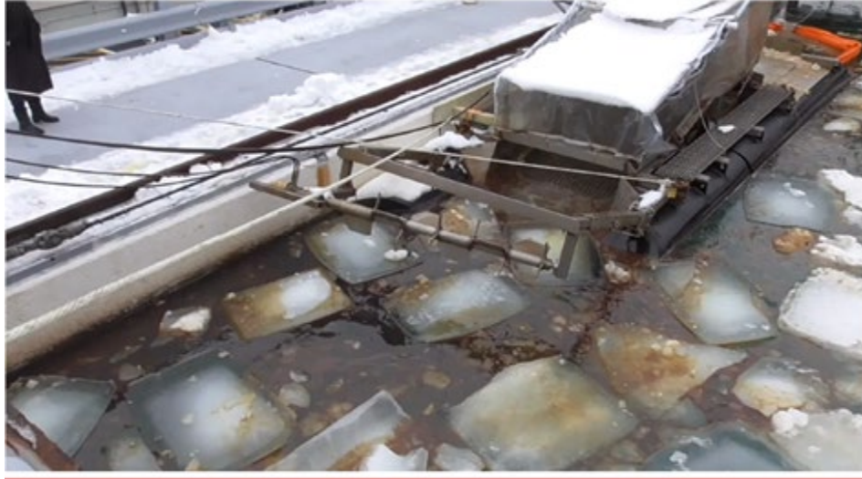
BOWHEAD ENCOUNTERING OIL AND ICE AS IT TRAVELS DOWN THE TEST TANK DURING 2021 TESTING (SOURCE: BSEE/OHMSETT, WITH PERMISSION)
