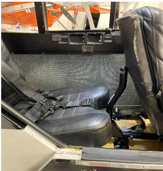
Figure 3 and Figure 4 shows the incorrectly installed aft control stick contacting the front pilot's seatback.
