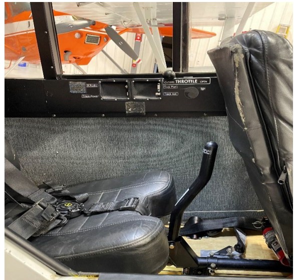
Figure 2 shows the aft control stick installed incorrectly.
