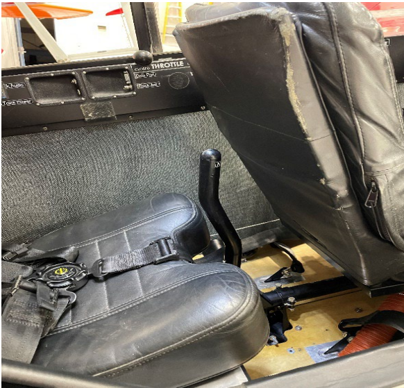
Figure 1 shows the control stick installed correctly allowing free range of travel.
