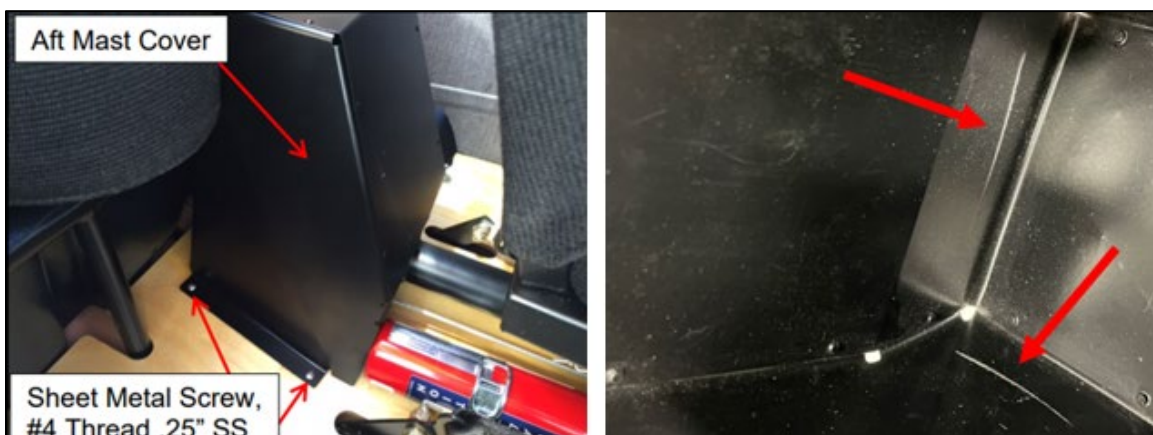
Figure 1. (Left) Proper Rear Stick cover installation. (Right) Scrape marks on the inside cover due to improper installation.
