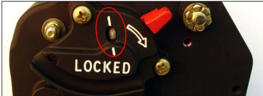
Figure 1. Some cargo hooks have sight window that will allow the user to see a hook lock indicator
