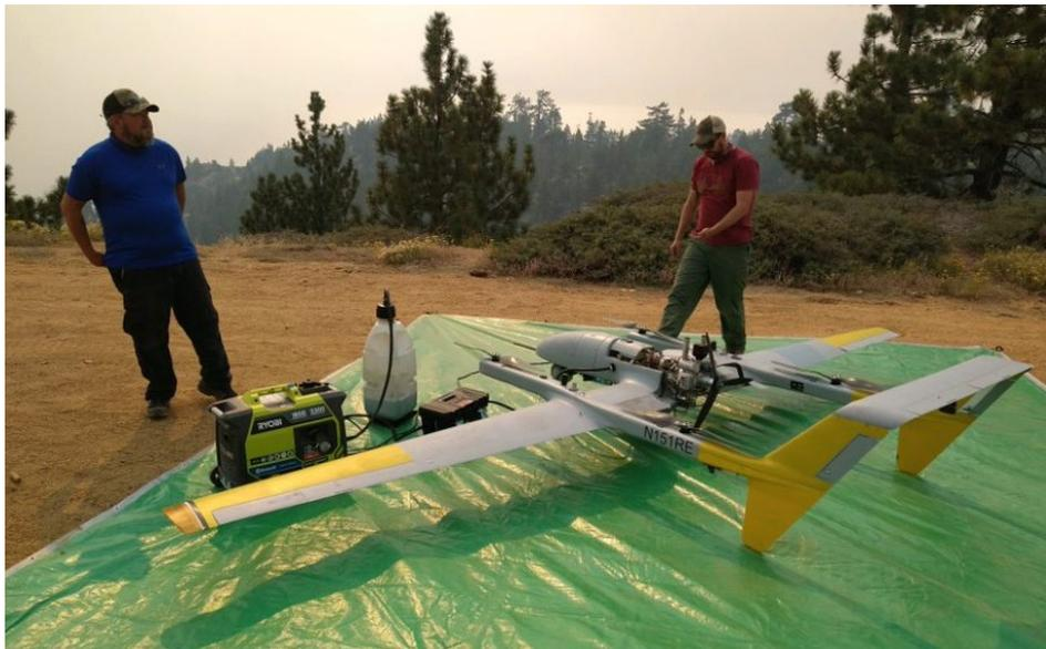
Bridger Aerospace’s Latitude FVR-90 “Type 2” unmanned aircraft conducted more than 60 flights in support of wildland fire operations in Fiscal Year 2020 as part of Interior’s CWN contract.
