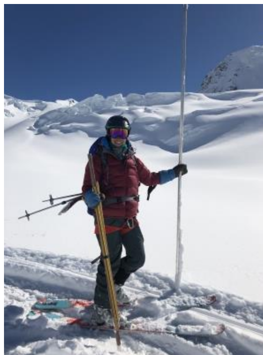
Researcher holds an ablation stake and winter snow probe during spring mass balance field work on Gulkana Glacier, AK. Source: USGS.
