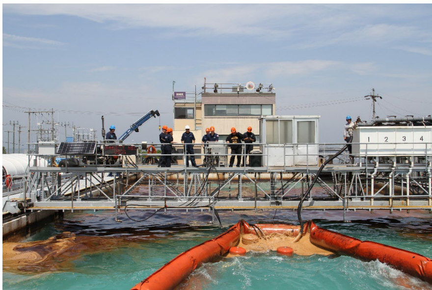
Figure 3. U.S. Coast Guard Strike Team personnel train on recovering oil with a skimmer in the Ohmsett tank. The USCG is an important customer for Ohmsett’s services.
