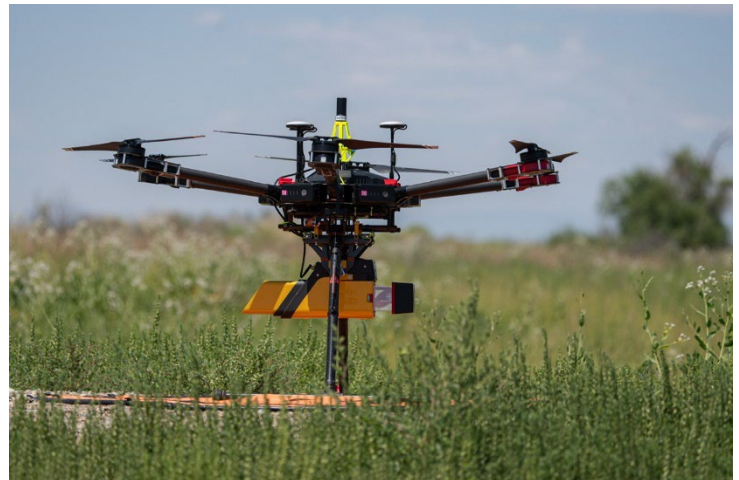
Figure 1 M600 UAS with a Yellowscan VX20-100 lidar scanner.
