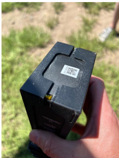
Figure 2 Cracked M600 Pro battery case.
