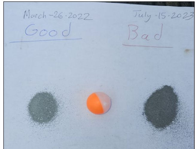
Figure 2 – The photo displays potassium permanganate. On the left side, it is depicted in its normal, lighter shade. On the right side, the potassium permanganate appears darker, indicating it has been affected.
