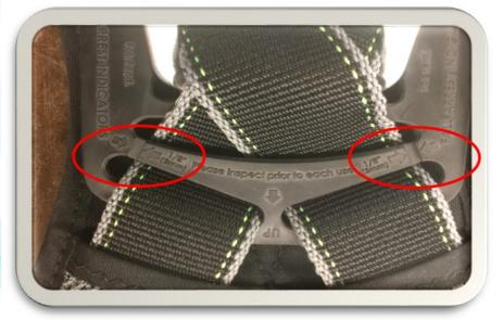
The points circled on the Fall Arrest Indicator (left) also need to be inspected prior to each use.
