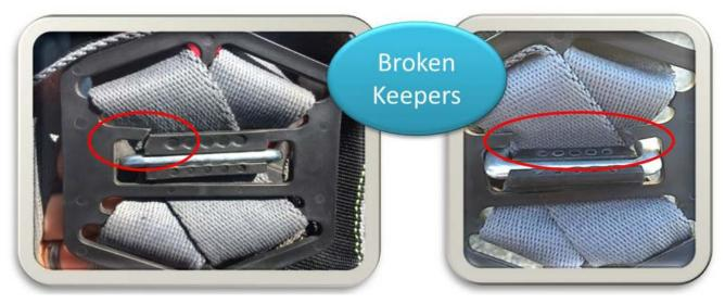
In Forest Service rappel operations, there are approximately 80 harnesses in service ranging in manufacture dates from 2006 through 2015. Most of the damage noted on these harnesses has occurred on harnesses manufactured before 2008. Although the manufacturer does not have a specific time life on their harnesses, the industry standard is 10 years. Harnesses over that time life should be retired.
