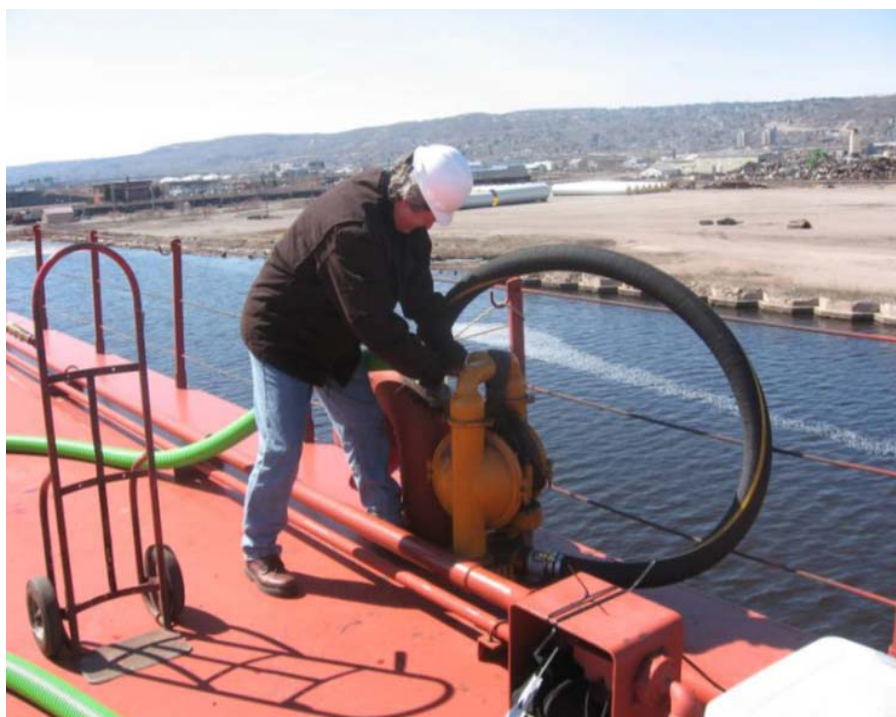
USGS's Dr. Barnaby Watten on the deck of American Steamship Company's Indiana Harbor testing passive nozzle mixing methods and gathering base line data. Dr. Watten is utilizing a diaphragm pump in order to pump water from one end of the ballast tank to the other in order to enhance the ballast mixing. [Photo Credit: Noah Adams, USGS]
