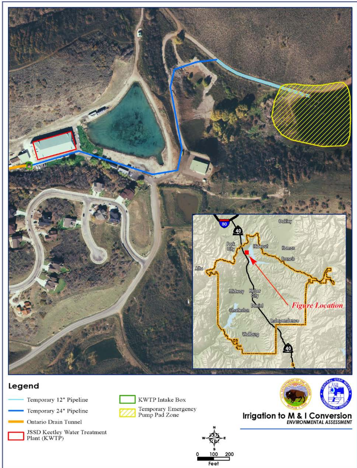
Figure 1-2. Temporary Pipeline and Pumping Station
