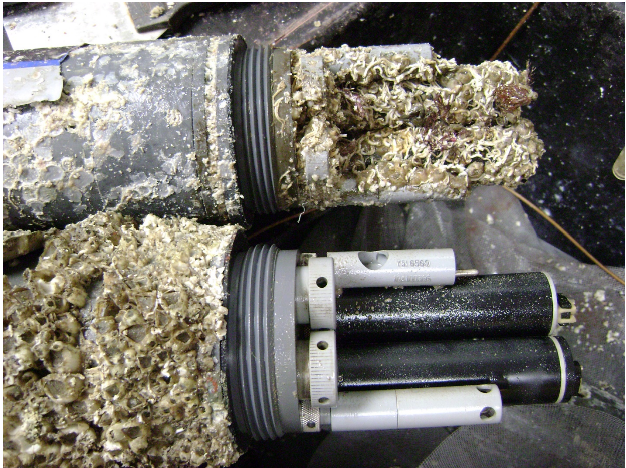
Two water quality instruments deployed side by side at Padre Island National Seashore showing the extent of biofouling without the invention (above) and with the invention (below). [Photo: Joe Meiman, NPS]
