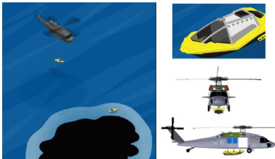
Conceptual illustrations of the remotely operated unmanned surface vehicle (ROUSV) being deployed to an oil slick via a helicopter. Credit: ExxonMobil.
