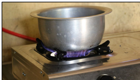
Working biogas digester cookstove Source: Northern Rangelands Trust
