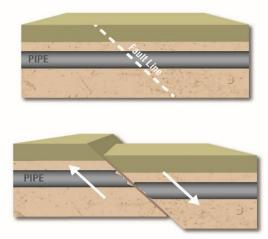
Figure 1-5. Illustration of Vertical Displacement.
