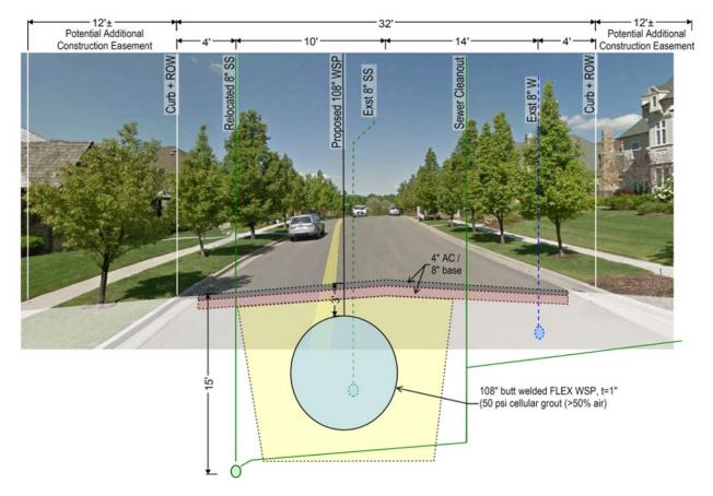
Figure 3-1. Cross-Section View of 1060 North.
