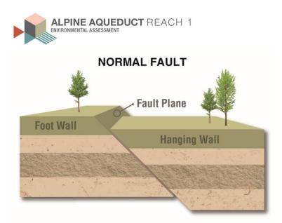
Figure 2-1. Hanging Wall and Foot Wall of a Normal Fault.
