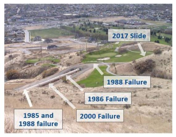
Figure 1-6. Pipeline Failures in the Last 40 Years.
