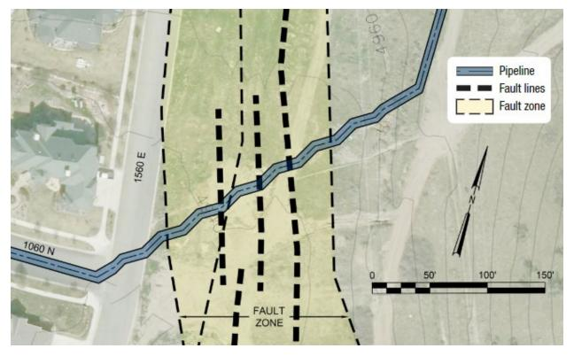
Figure 2-3. Stacked Pipe Design for Fault Crossings.
