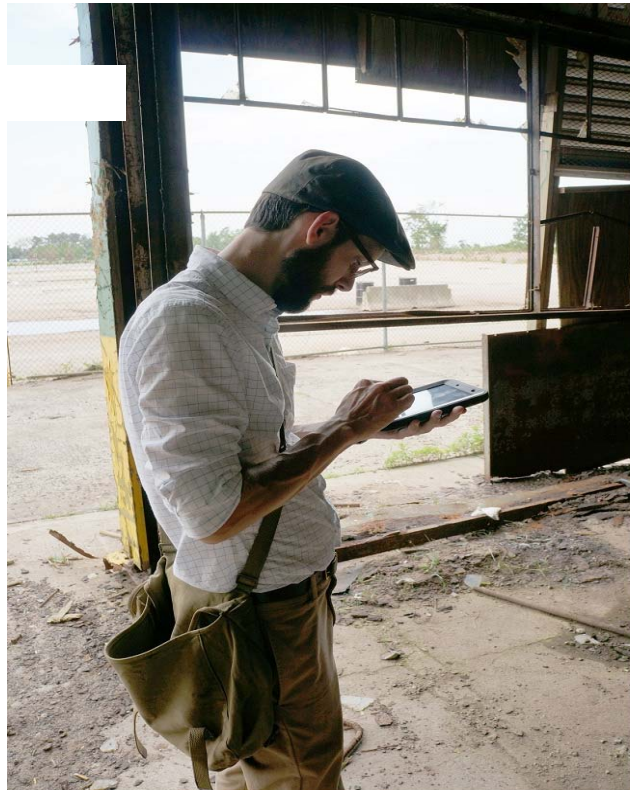
NPS contractor Ed FitzGerald surveys the interior of historic Seaplane Hangar #38 using a beta version of MoCA, NCPTT's mobile app for post-disaster condition surveys. Miller Army Airfield, Gateway NRA, Staten Island, NY, Superstorm Sandy recovery, June 2013. Photo: NPS.
