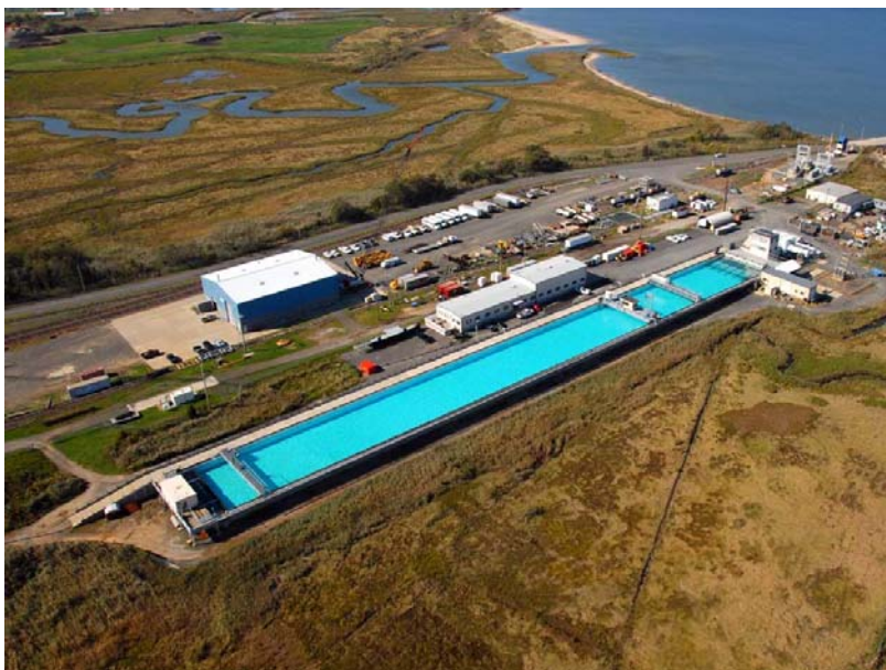
The Ohmsett facility in Leonardo, NJ, at Naval Weapons Station Earle Waterfront. The 2.6 million-gallon salt water tank in the foreground is used to test full scale oil spill response technologies and to train response personnel from other government agencies (e.g., U.S. Coast Guard and the Navy), private industry and other non-governmental organizations. More than twenty-four countries have conducted tests or training at the Ohmsett facility. Photo credit: BSEE.
