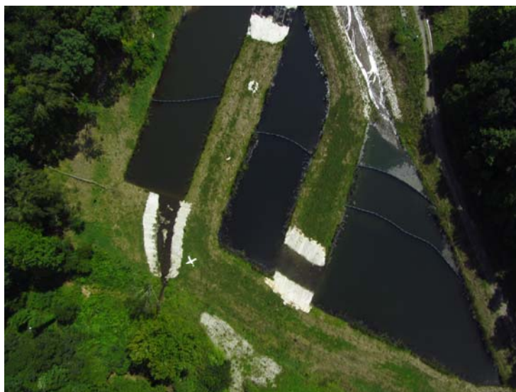
Oversight of mining activities: At 400 feet above the surface, the T-Hawk, an Unmanned Aerial Vehicle (UAV), captures an image of drainage control ponds constructed at the Hobet 21 surface coal mine complex, near Danville, Boone Co, West Virginia. The complex is operated by Hobet Mining Inc. Photo: OSMRE
