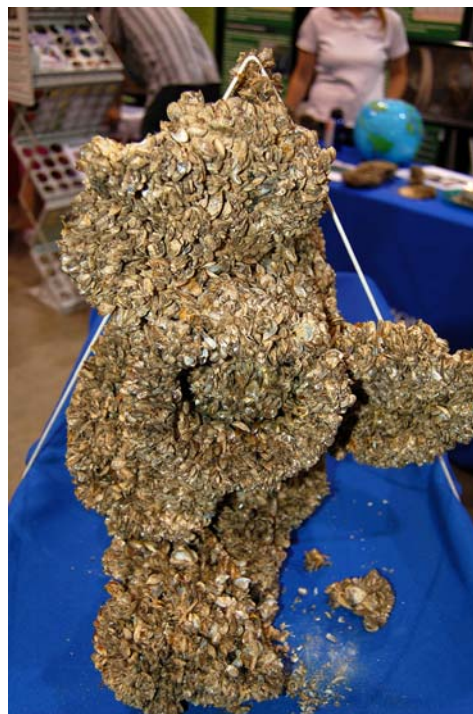
Outboard motor encrusted with quagga mussels. Photo: Neal Muirhead, Bureau of Reclamation.
