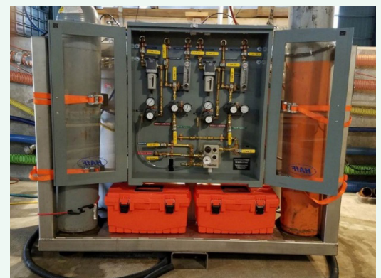
The USGS Hyperbaric Apparatus for Fish used to assess barotrauma in Great Lakes fishes. Photo credit: Owen Gorman, USGS
