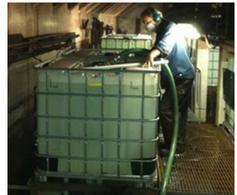
Barnaby Watten adding sodium hydroxide to a ballast water test chamber aboard the Motor Vessel (M/V) American Spirit . Photo credit: USGS
