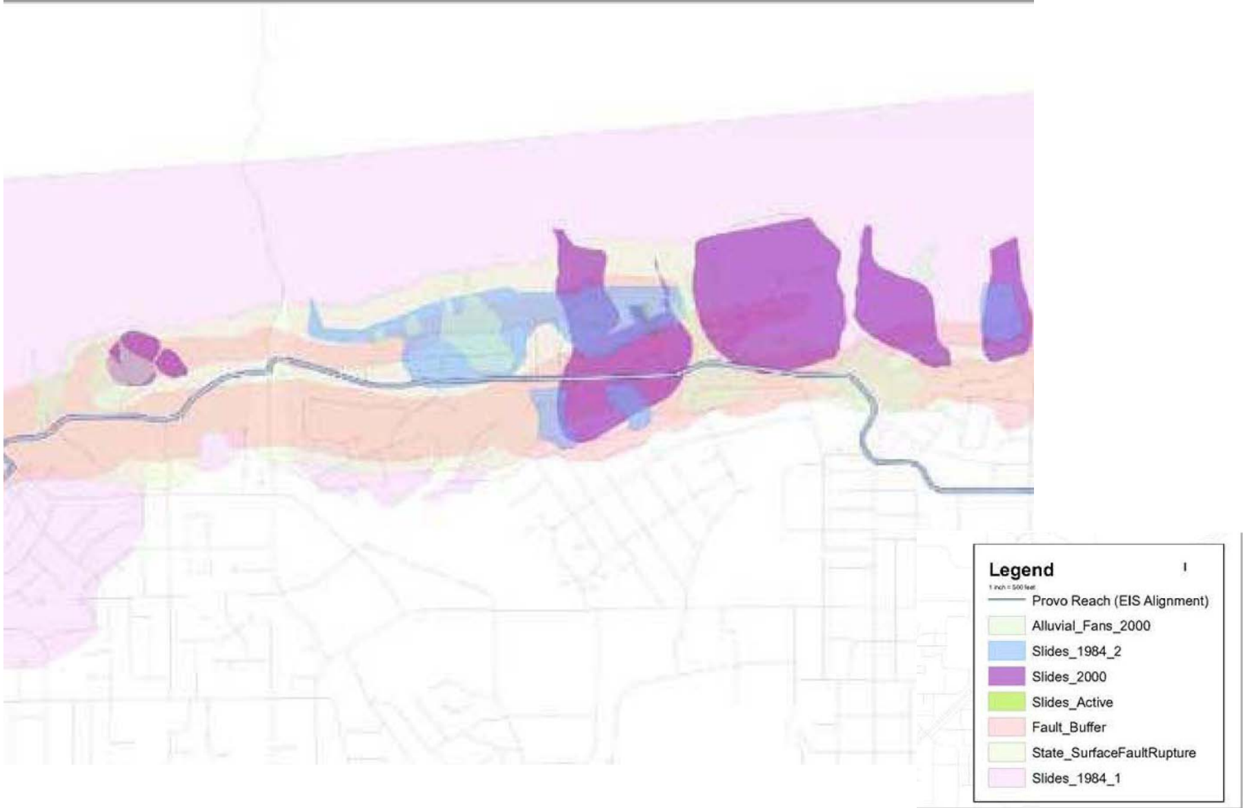
Figure 1: UAGRS data for landslides and faults along DPR Stations 675+00 to 764+00.
