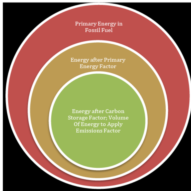
Figure A17. Determining quantities of energy to multiply by emissions factor
