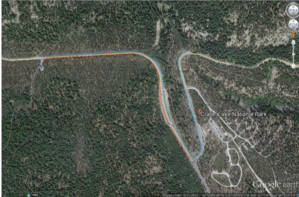
Figure 4. Alternative alignments considered of water, power and communication lines from the PCT Well to Existing Munson Valley Water Distribution Line utilizing existing highway corridor.
