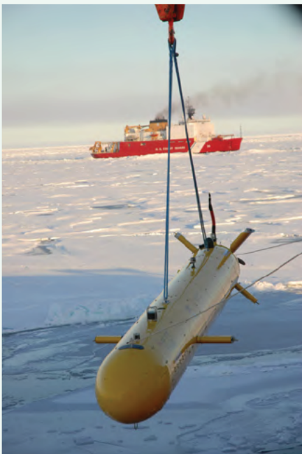
The autonomous underwater vehicle (jointly developed by Defense Research and Development Canada and International Submarine Engineering, Ltd) being deployed from the Louis as the Healy is seen in the background. Photo credit: Debbie Hutchinson
