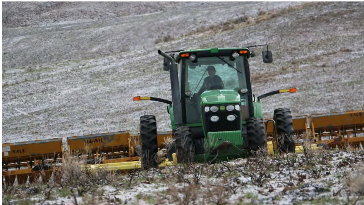
Rangeland drill restoration after Soda Fire
