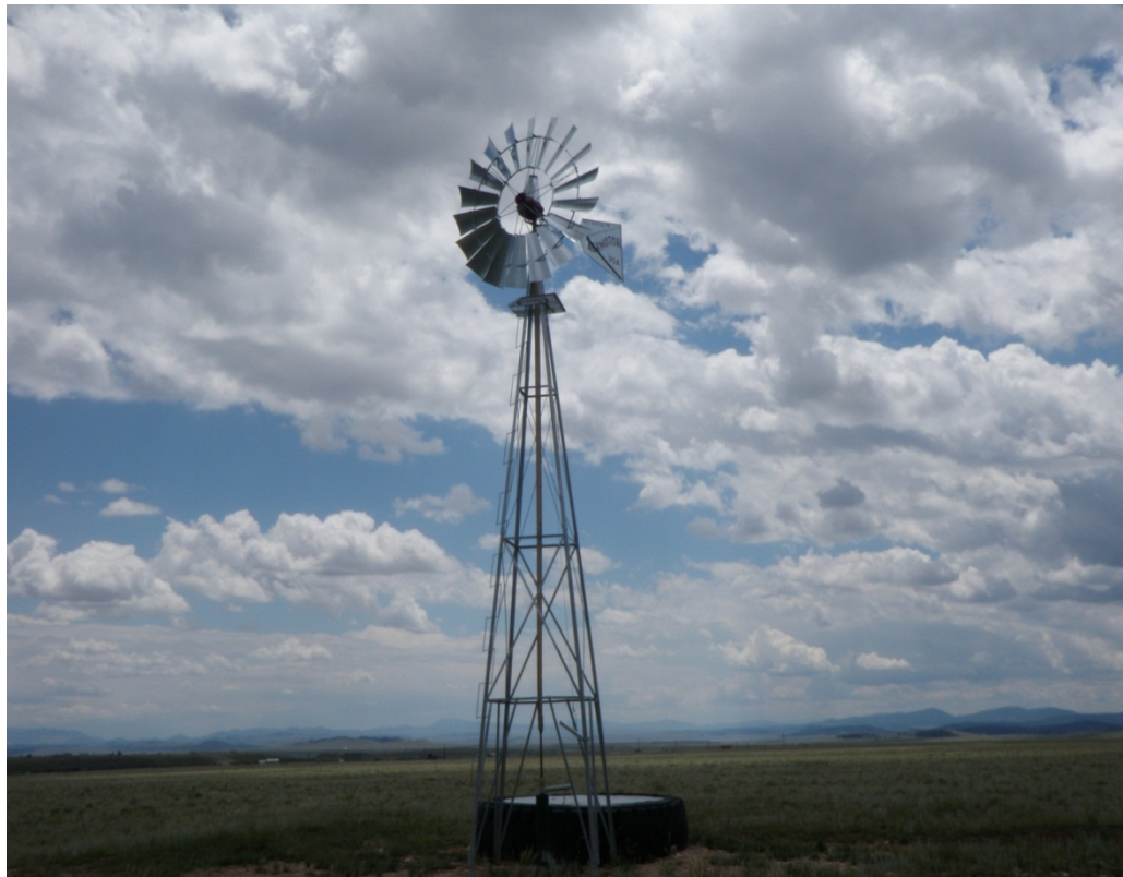
A windmill powered well is used to improve livestock distribution in Colorado in an area without a reliable water source.
