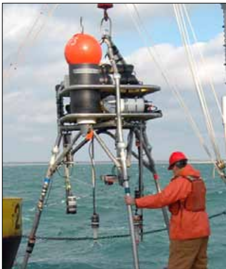
USGS scientists deploying instrument tripod to the seafloor. Photo credit: Sandy Baldwin, USGS.
