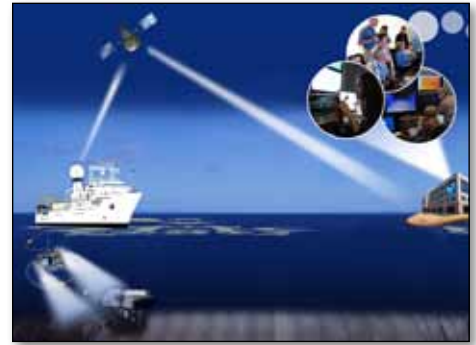
NOAA Ship Okeanos Explorer uses satellite technology to transmit data and video in real-time from the ship and ROVs working at depth, to a shore-based hub where the video is transmitted in high definition out on Internet2 to a variety of receiving stations on shore. This telepresence allows scientists located on shore to join the operation in real-time. Image credit: NOAA Okeanos Explorer Program
