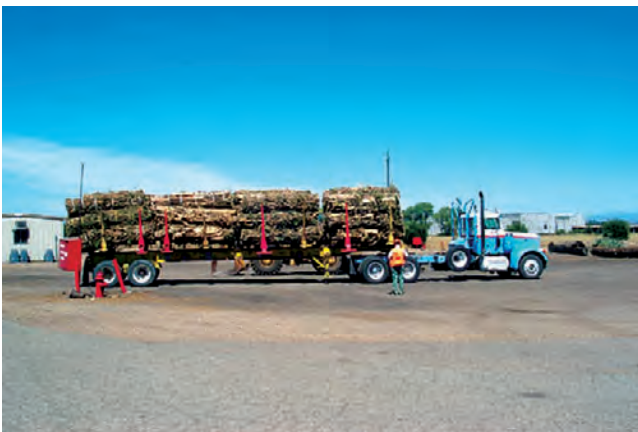
Figure 4. Log truck loaded with slash bundles for transport to a bioenergy facility. From Rummer and others (2004); U.S. Forest Service photograph.
