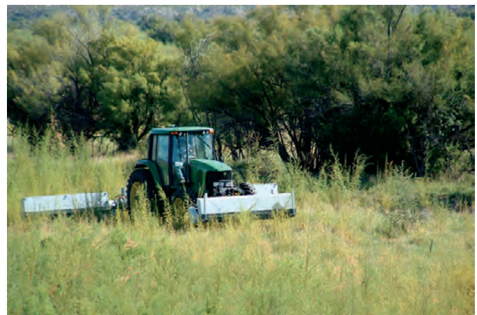
Figure 11. A 24-foot (approx. 8 m) carpet roller. Photograph by B. Tanzy, Bureau of Reclamation.
