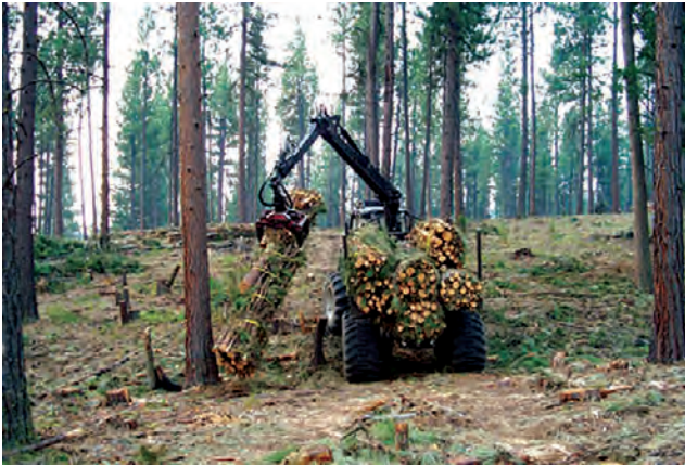
Figure 3. Forestry forwarder collecting slash bundles for transport to a roadside landing. From Rummer and others (2004); U.S. Forest Service photograph.
