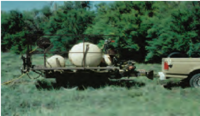
Figure 12. Low-pressure, moderate-volume ground sprayer mounted on a trailer. From Sisneros (1994).
