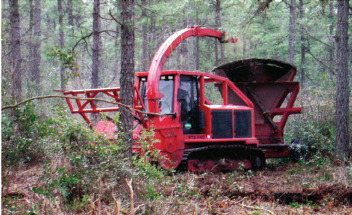
Figure 5. Modified forest mulching machine developed by North Carolina State University in cooperation with FECON, a producer of forestry machines. The modified mulcher shown here includes a device to blow ground particles into a trailer towed behind the mulching vehicle. From Livingston (2008).
