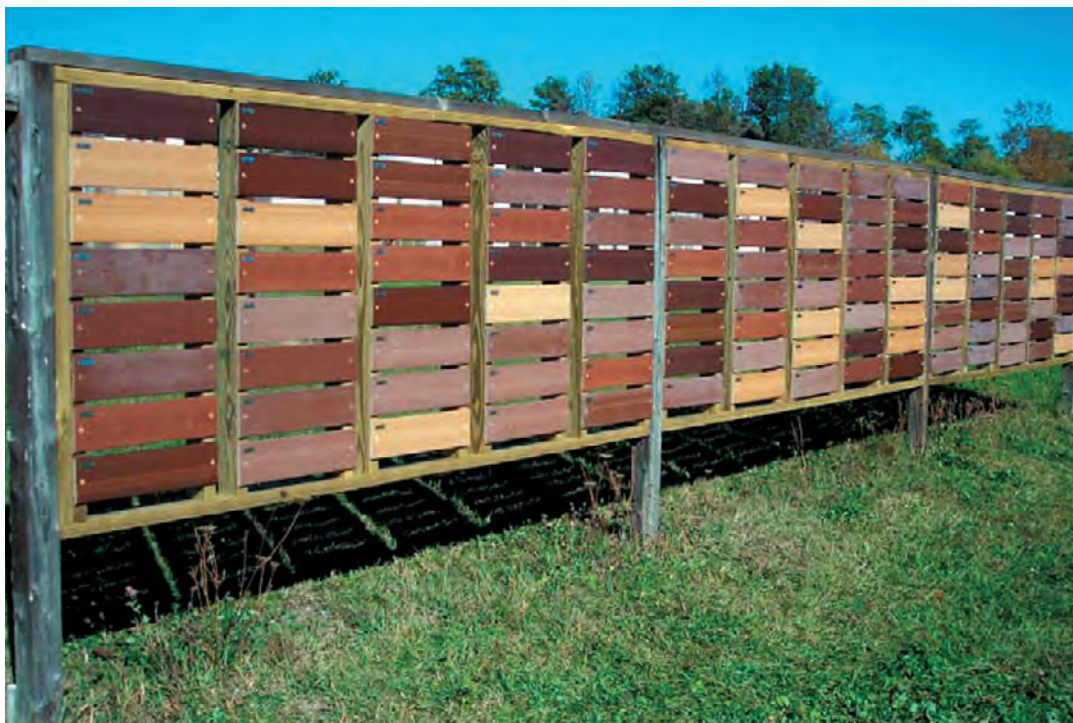
Figure 6. Natural weathering test rack with extruded composite boards manufactured from saltcedar-, juniper-, and pine-wood flours. Saltcedar boards are those with the darkest coloring. From Stark and Clemons (2008); U.S. Forest Service photograph.
