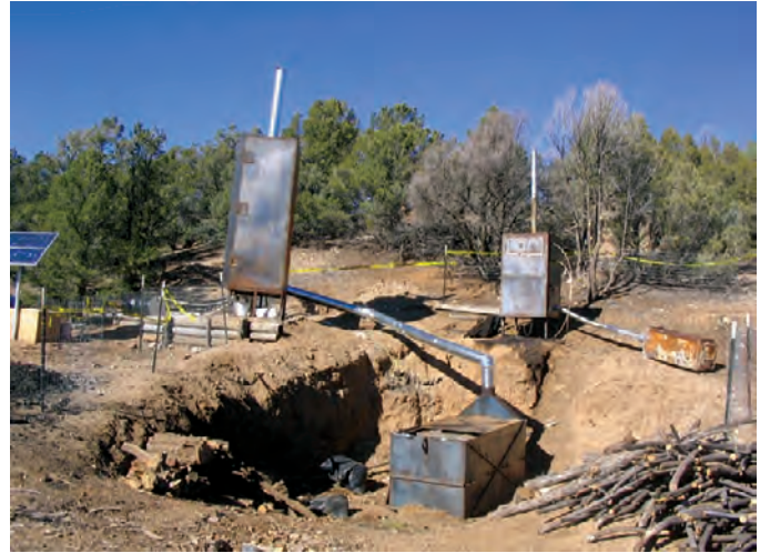
Figure 7. Field setup for charcoal production in the project described by Taylor (2005). At left is a solar panel used to power a water pump for the wood-preservation chambers. The pickup-truck-transportable charcoal kiln is located in the pit, with exhaust gases piped to a tall wood-preservation chamber to the left of and behind the kiln. At right rear are a smaller charcoal kiln and preservation chamber for short wood pieces. Photograph copyrighted by Lynda Taylor, used with permission.
