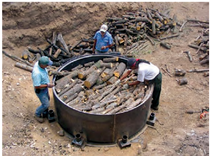
Figure 8. The large kiln being charged. Several species of wood were included in each charge but segregated within the kiln to facilitate testing. Photograph copyrighted by Lynda Taylor, used with permission.
