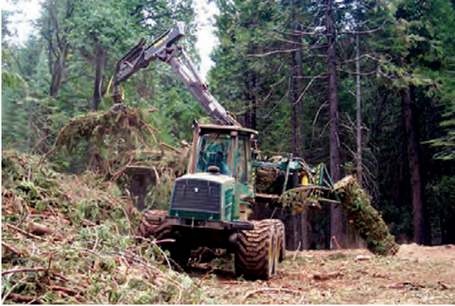
Figure 2. The John Deere 1490D Slash Bundler in operation. In the photograph, one of the twine-wrapped cylindrical bundles produced by the machine has just been released. From Rummer and others (2004); U.S. Forest Service photograph.
