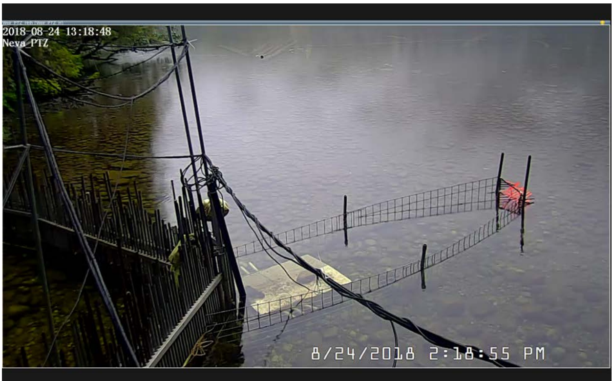
Figure 2. Screen capture of surveillance video feed from the Neva Lake weir, showing the beaver-deterrent fence around the video chute.
