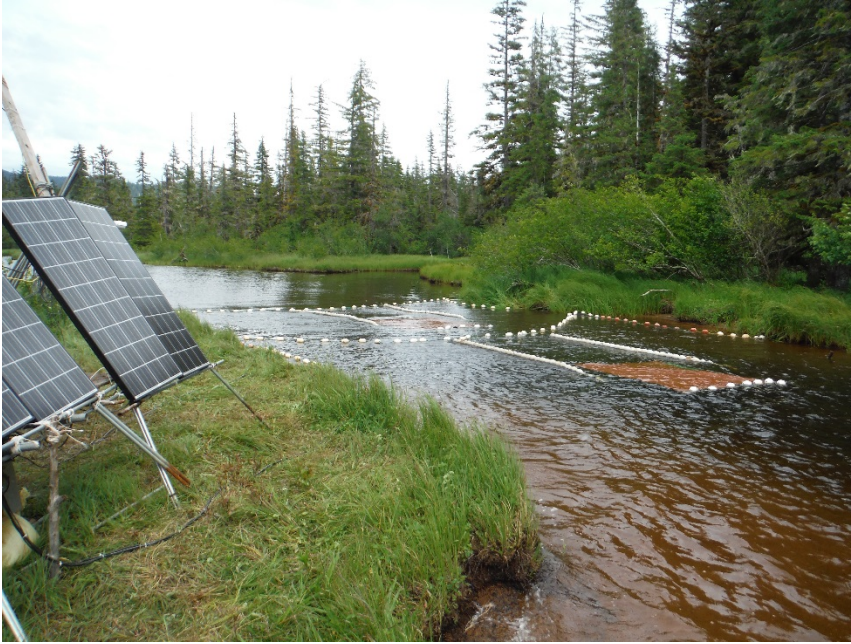
Figure 1. Video weirs at the outlet of Sitkoh Lake, 2017
