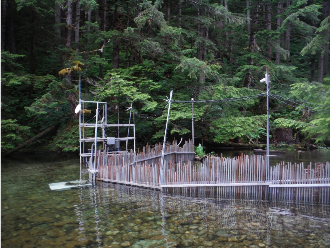
Figure 1. The remotely monitored video weir at Neva Lake, near Excursion Inlet.
