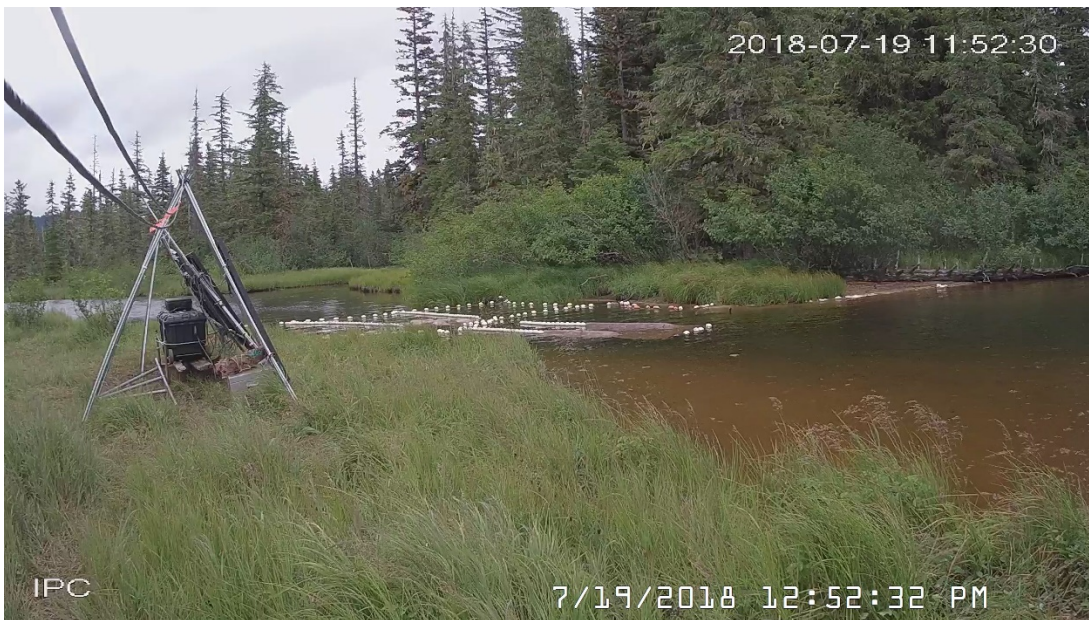
Figure 3. Live video capture from a surveillance camera at the Sitkoh Lake video weir.
