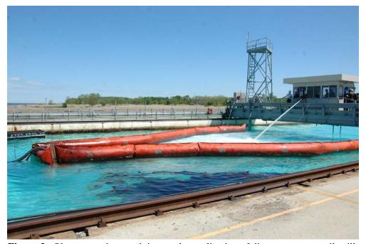
**Figure 2**. Ohmsett students training on the application of dispersants to an oil spill.
