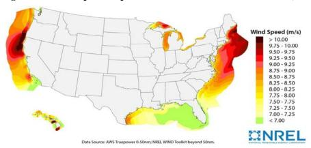
Figure 12: Wind Speed Map for the U.S. Technical Resource Area (100m Height)
