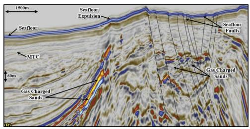
Seismic Data Showing Shallow Geohazards
