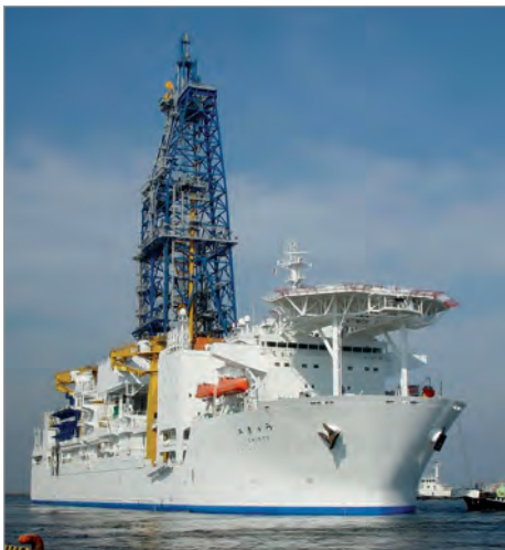
The deepwater vessel Chikyu as deployed during the second joint Indian National Gas Hydrate Program Expedition 02. The vessel was designed by the Japanese government for international scientific drilling operations. Photo credit: Japan Agency for Marine-Earth Science and Technology
