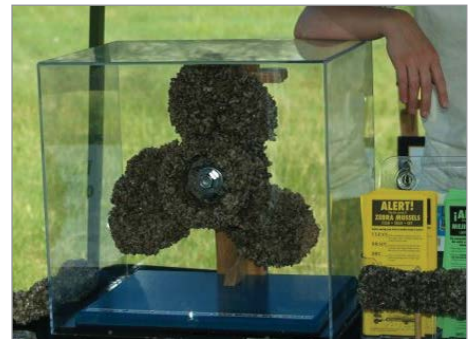
A display of invasive zebra mussels shows how they can propagate and foul propellers and clog pipelines. Photo credit: USFWS
