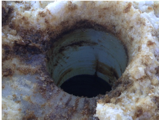
Figure 3.2. An auger hole drilled to recover oil by “auger ice mining.” Layers of oil-contaminated ice are visible in the photograph, suggesting that oil may have become trapped within ice layers and fissures as the river water froze during cold conditions in the days after the spill.
