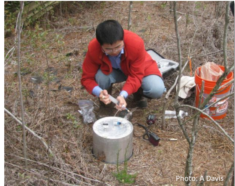
Measuring GHG benefits of wetland restoration at Pocosin Lakes NWR
