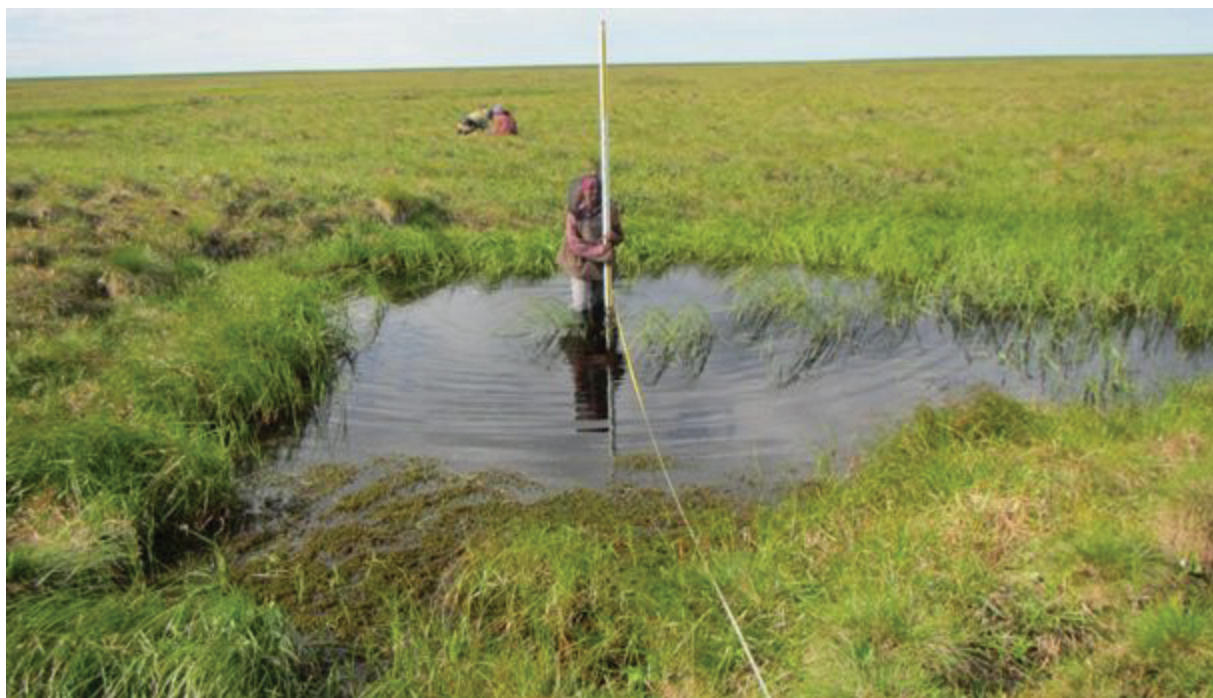
Figure 9. Topographic surveys through thermokarst terrain document changes in landforms due to permafrost thawing and refreezing.
