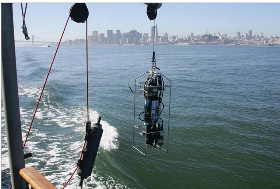
Instruments used to measure a variety of water quality constituents are deployed off the ship's boom, with the San Francisco skyline in the background. Photo credit: USGS
