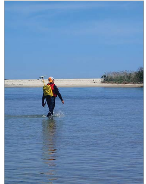
USGS scientist Owen Brenner walks across the Fire Island wilderness breach carrying a GPS backpack that allows him to collect precise elevation data in the shallows. Photo credit: Cheryl Hapke, USGS
