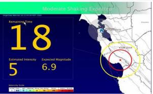
Figure 1: The ShakeAlert UserDisplay shows the user's location (house symbol), earthquake epicenter (red dot), P waves (yellow circle), S waves (red circle), estimated magnitude (6.9), estimated intensity (5), and remaining time until the shaking is expected to start (18 seconds) (Source: https://www.shakealert.org/).
